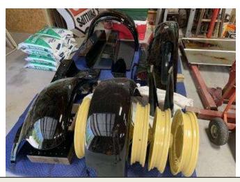
Fenders, splash guards, and running boards back from paint shop. Wheels also powder coated.
